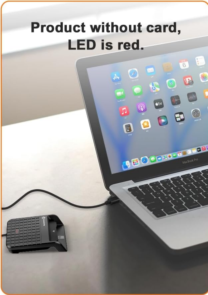
Image 4.2.1: Comparison showing the smart card reader's LED status: red when no card is present, and green/red when a smart card is inserted and detected.
