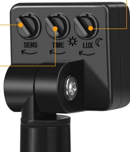
Figure 3: Close-up of the motion sensor with its three adjustable modes: SENS (sensitivity), TIME (lighting duration), and LUX (day/night setting).
