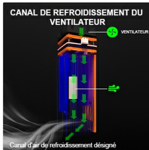
Figure 5.3: Fan Cooling Channel. This diagram illustrates the designed air cooling channel with a fan, ensuring efficient heat dissipation for the laser module.
