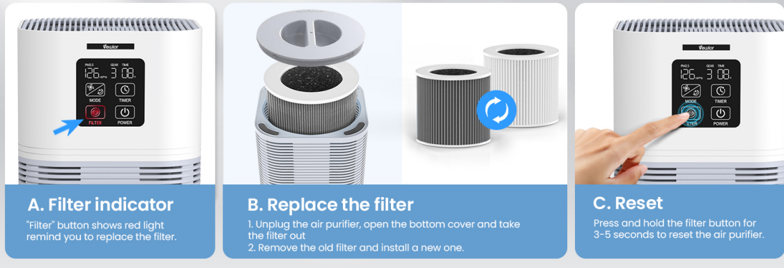
Figure 4: Visual guide for filter replacement and reset.
