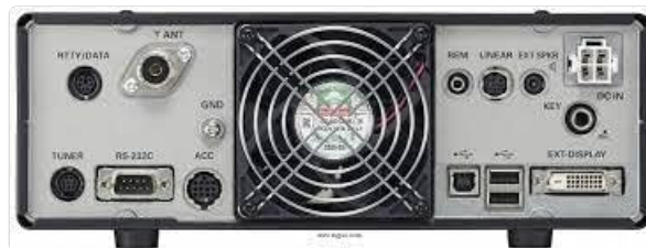
Figure 2: Rear view of the Yaesu FTDX-10 HF Transceiver, displaying antenna connectors, power input, and various accessory ports.
