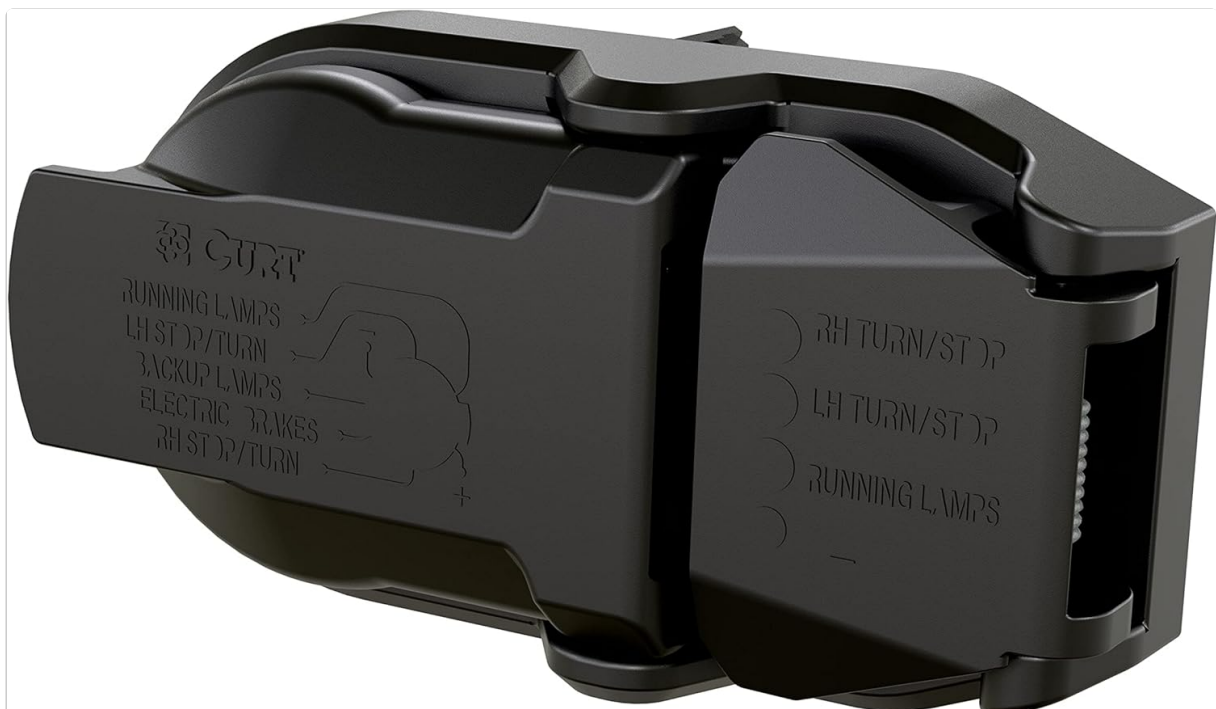
Image: The CURT 57015 dual-output connector, showing the 7-pin and 4-pin sockets. The 7-pin side indicates connections for running lamps, left stop/turn, backup lamps, electric brakes, and right stop/turn. The 4-pin side indicates
