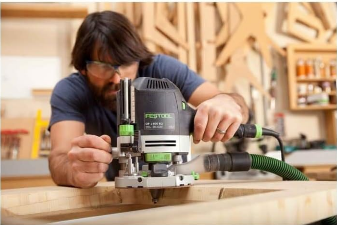
Figure 4.3: A user operating the Festool OF 1400 EQ-F-Plus Plunge Router, demonstrating the use of guide rods for controlled and precise routing along an edge.
