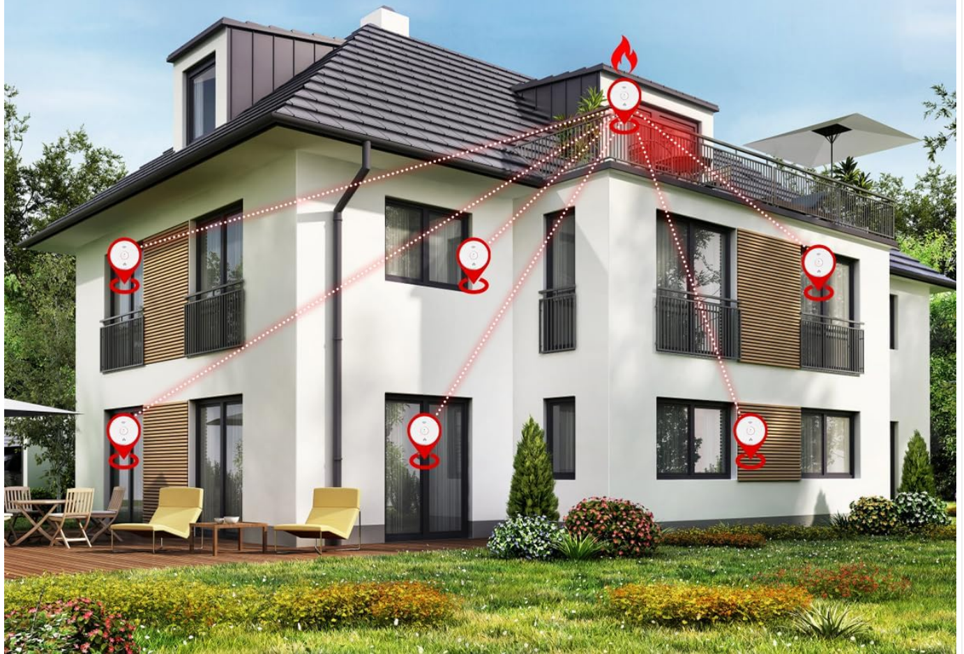
Figure 8: When one alarm detects danger, all interconnected alarms will sound.
