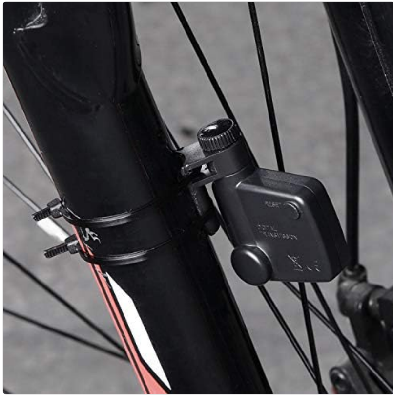
Image: The bike computer mounted on handlebars and the sensor/magnet on the fork.
