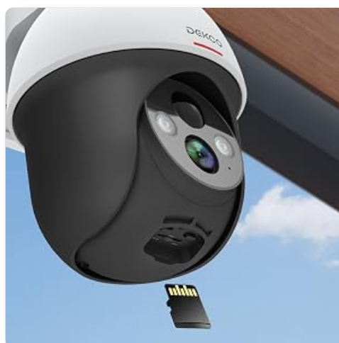
Figure 7: SD card slot for local storage.
