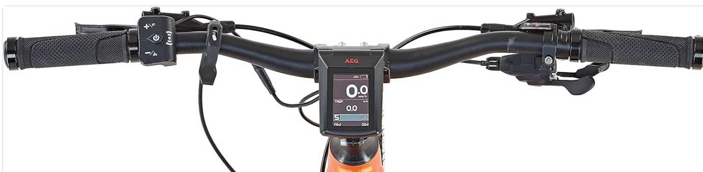
Figure 4: The AEG TFT display and handlebar controls, including the suspension lockout lever.
