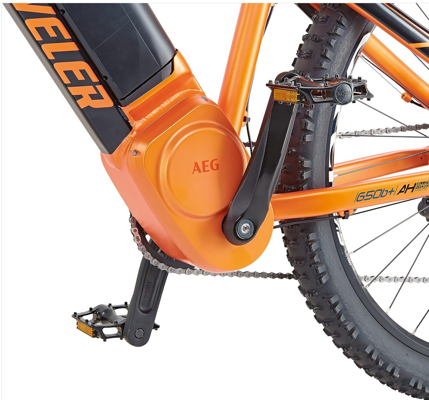
Figure 3: The AEG SportDrive central motor, providing powerful pedal assistance.
