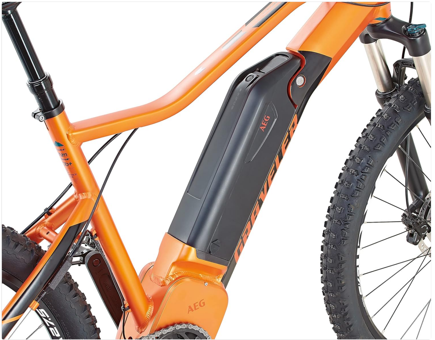
Figure 2: Close-up of the semi-integrated AEG DownTube battery.
