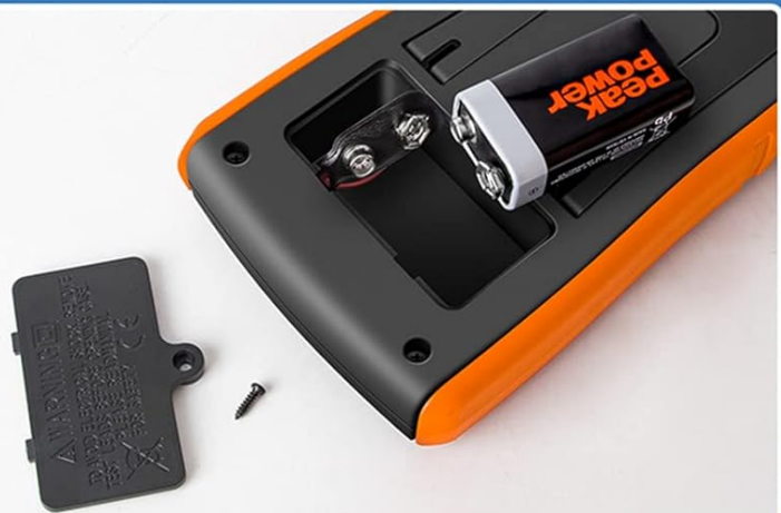
Figure 3: Battery installation. This image illustrates the process of installing a 9V battery into the multimeter's battery compartment, showing the correct polarity connection.
