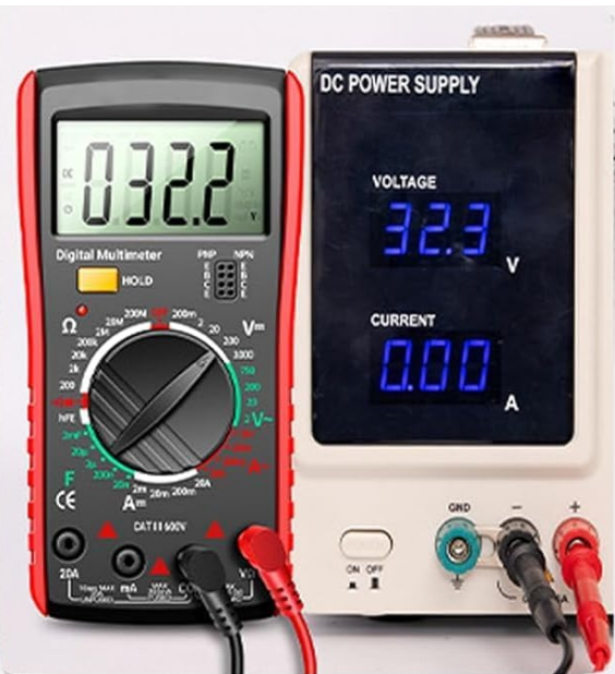
DC Voltage Measurement
