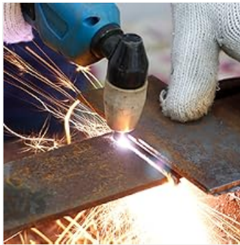
Figure 5.4: Example of plasma cutting in progress.
