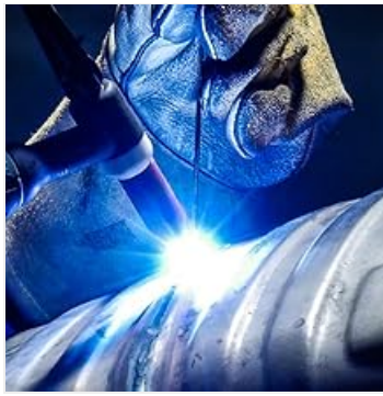
Figure 5.3: Example of TIG welding in progress.
