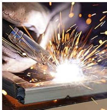
Figure 5.2: Example of MIG welding in progress.
