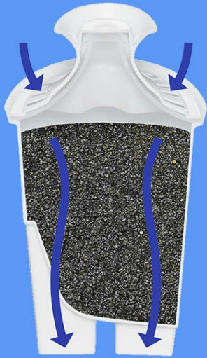
Figure 4: Brita Original filter technology, showing water flow through vents and mesh screens.
