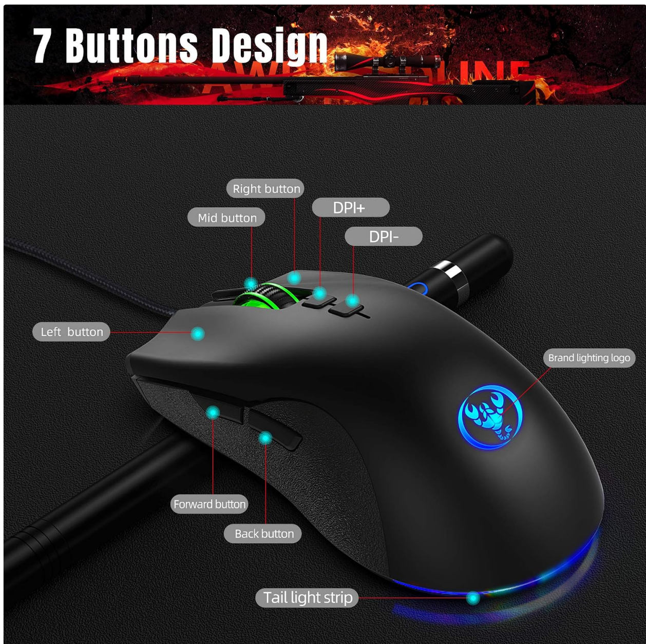
Figure 5.1: Labeled diagram of the 7 programmable buttons on the UINO A883 Gaming Mouse, including Left, Right, Mid, DPI+, DPI-, Forward, and Back buttons, along with the brand lighting logo and tail light strip.
