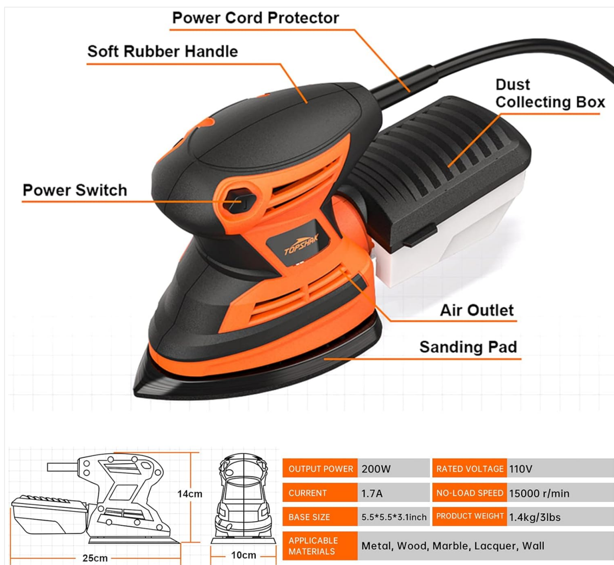
Figure 3.1: Key components of the sander, including the Power Cord Protector, Soft Rubber Handle, Power Switch, Dust Collecting Box, Air Outlet, and Sanding Pad.
