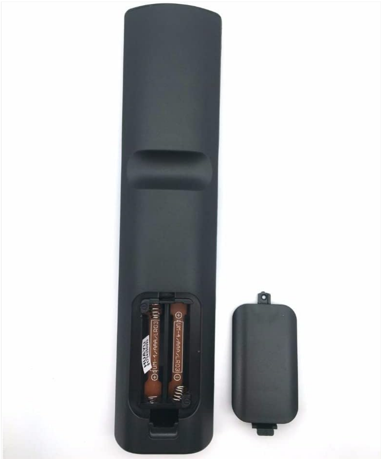
Figure 3.1: Back view of the remote control with the battery compartment open, showing the correct orientation for AAA battery insertion.
