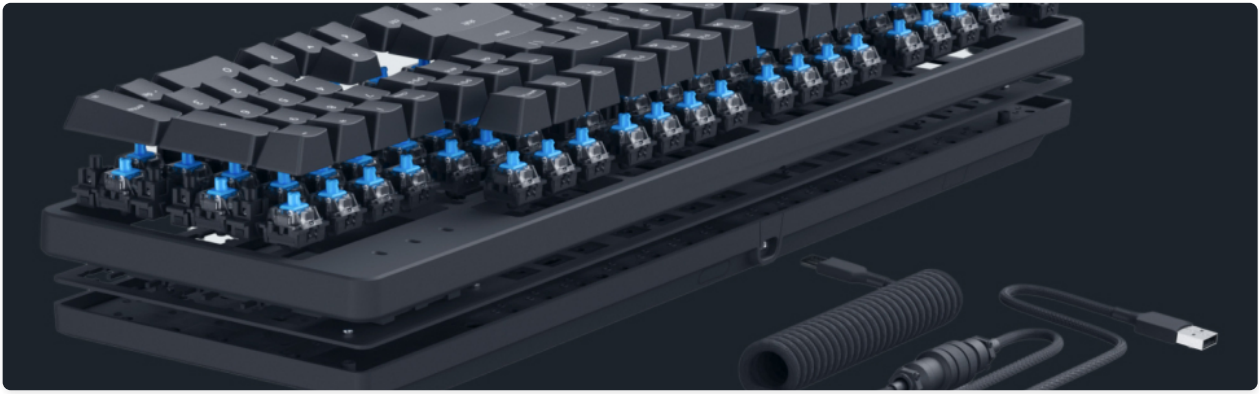
Image 4.5: The keyboard's modular design with swappable top cover plate, keycaps, and switches.
