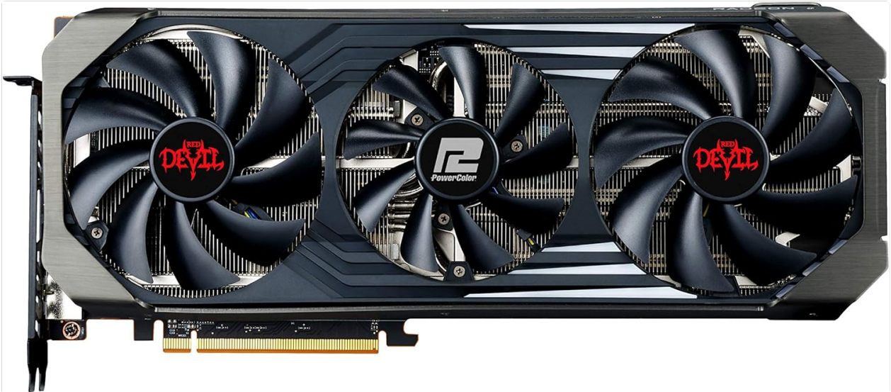
Image: Front view of the PowerColor Red Devil AMD Radeon RX 6750 XT Graphics Card, showcasing its triple-fan cooling system and Red Devil branding.
