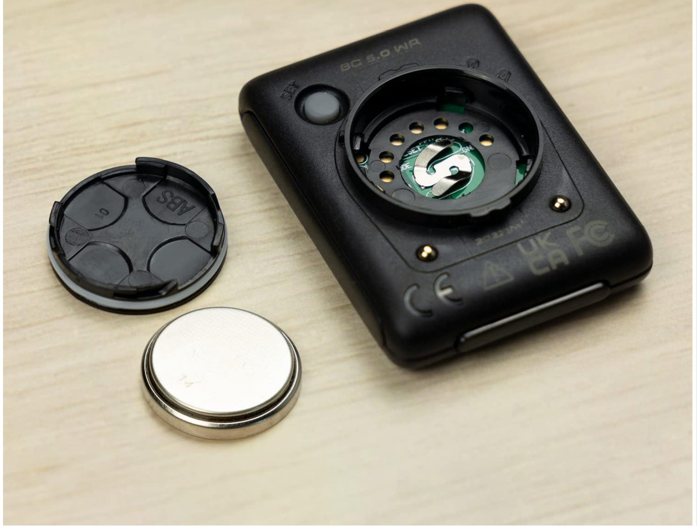
Figure 2: Battery Compartment. This image shows the rear of the Sigma BC 5.0 bike computer with the battery cover removed, revealing the CR2032 battery slot.
