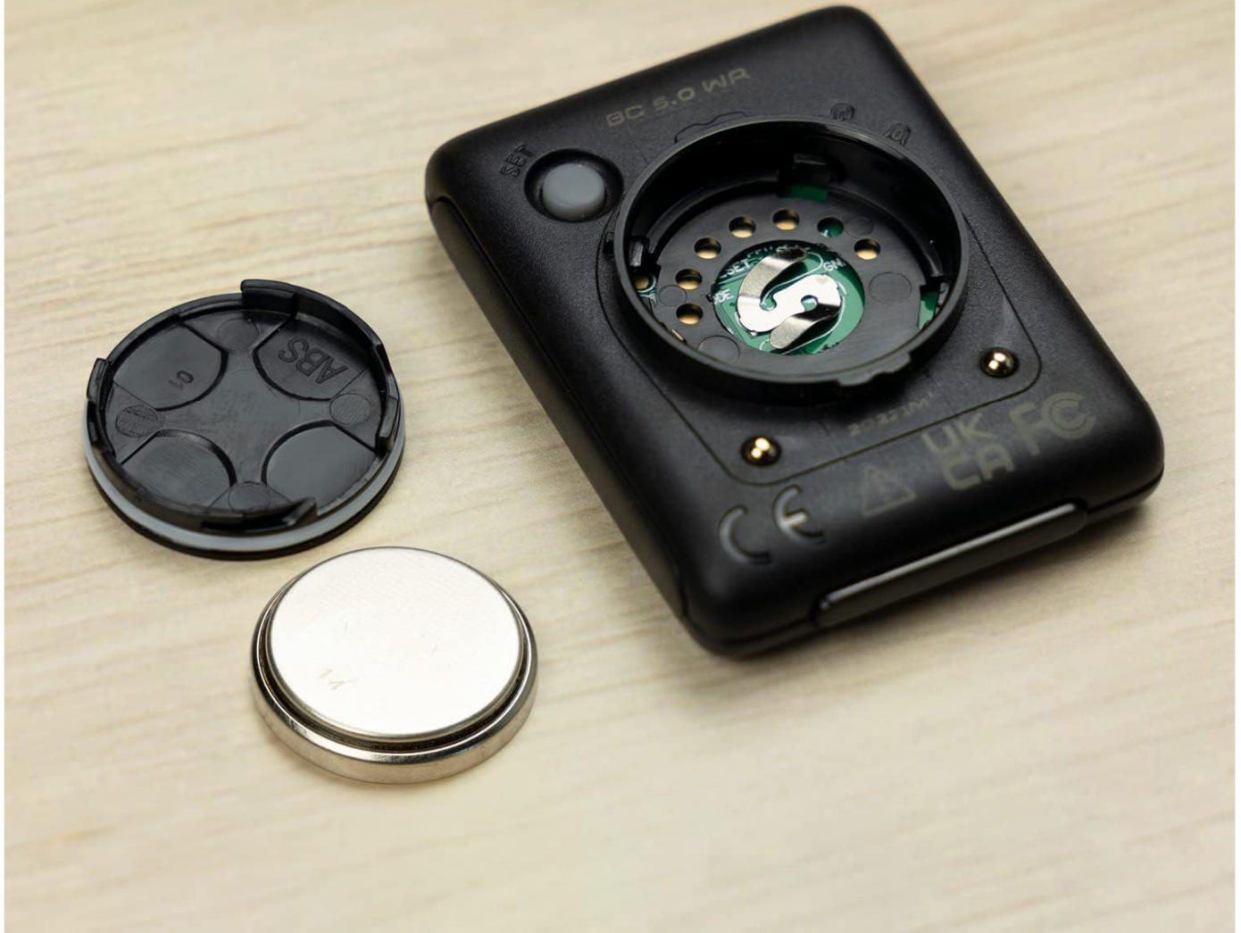
Image: View of the battery compartment on the rear of the Sigma BC 5.0, showing the CR2032 battery and its cover. The device is designed for a battery life of 2+ years.
