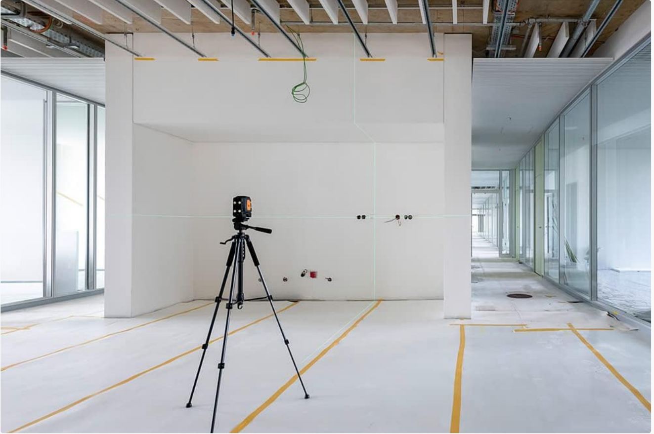
Figure 3: The GEO1X-GREEN laser positioned on a tripod in a spacious construction environment, demonstrating its use for establishing level lines across a wide area. The green laser lines are clearly visible on the walls.
