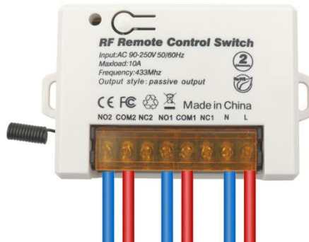
Figure 2: Details of the screw terminals and passive output relay.
