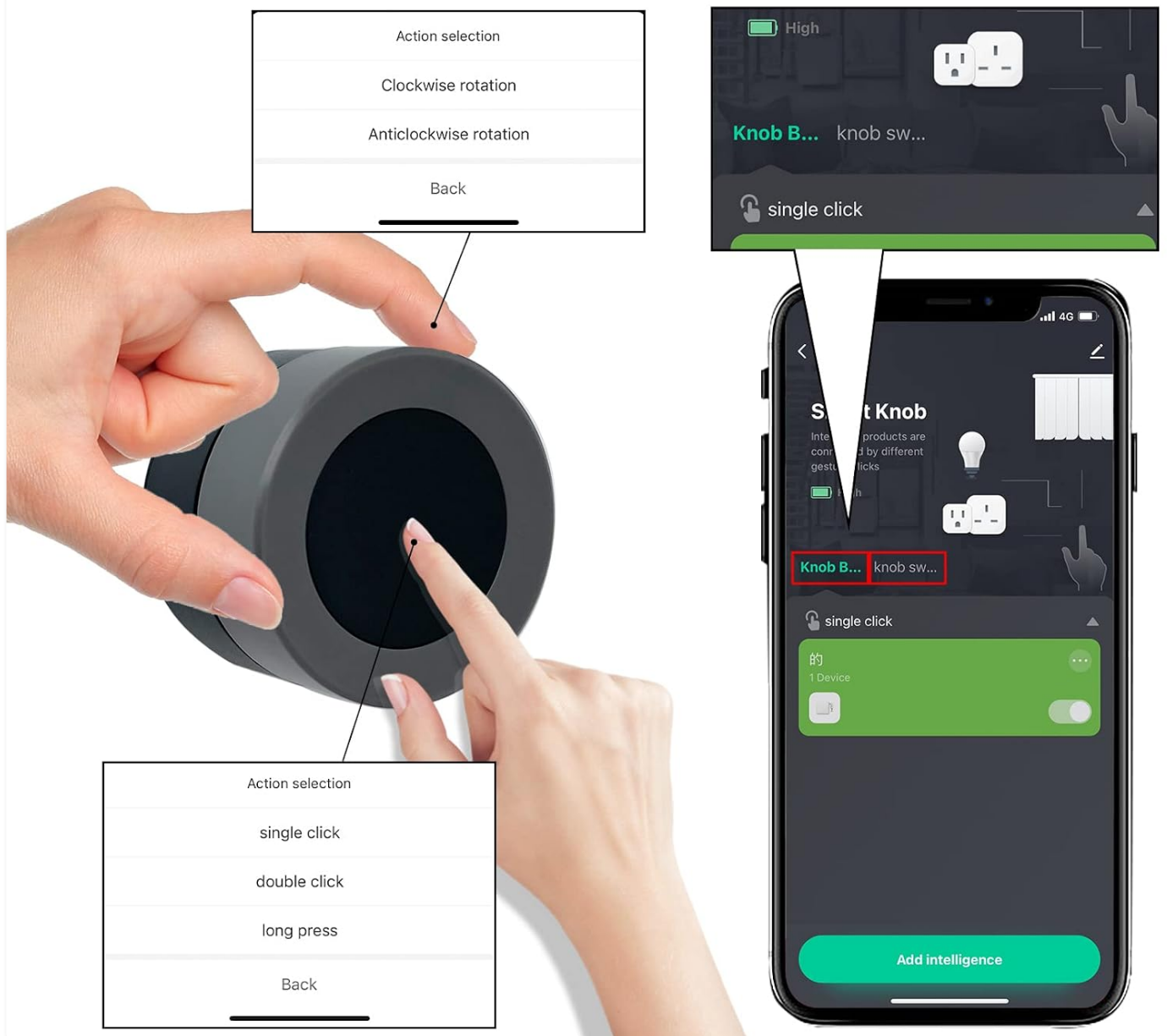
Figure 6: App interface demonstrating the configuration options for the knob button and switch actions within the Smart Life App (compatible with Tuya Smart App).
