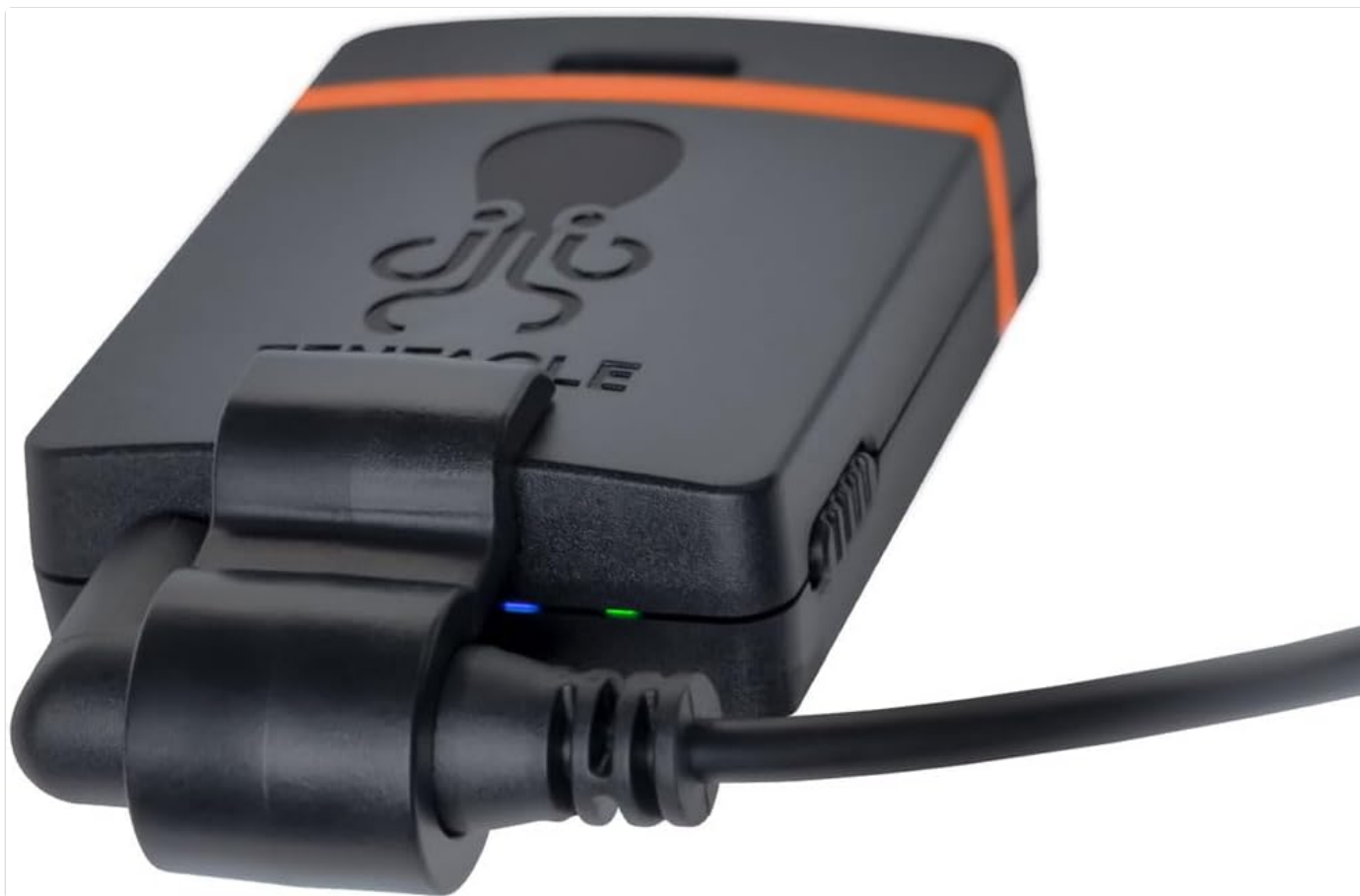
Figure 5.2: The Tentacle Sync E MKII with a 3.5mm mini-jack cable connected, ready for timecode input/output.
