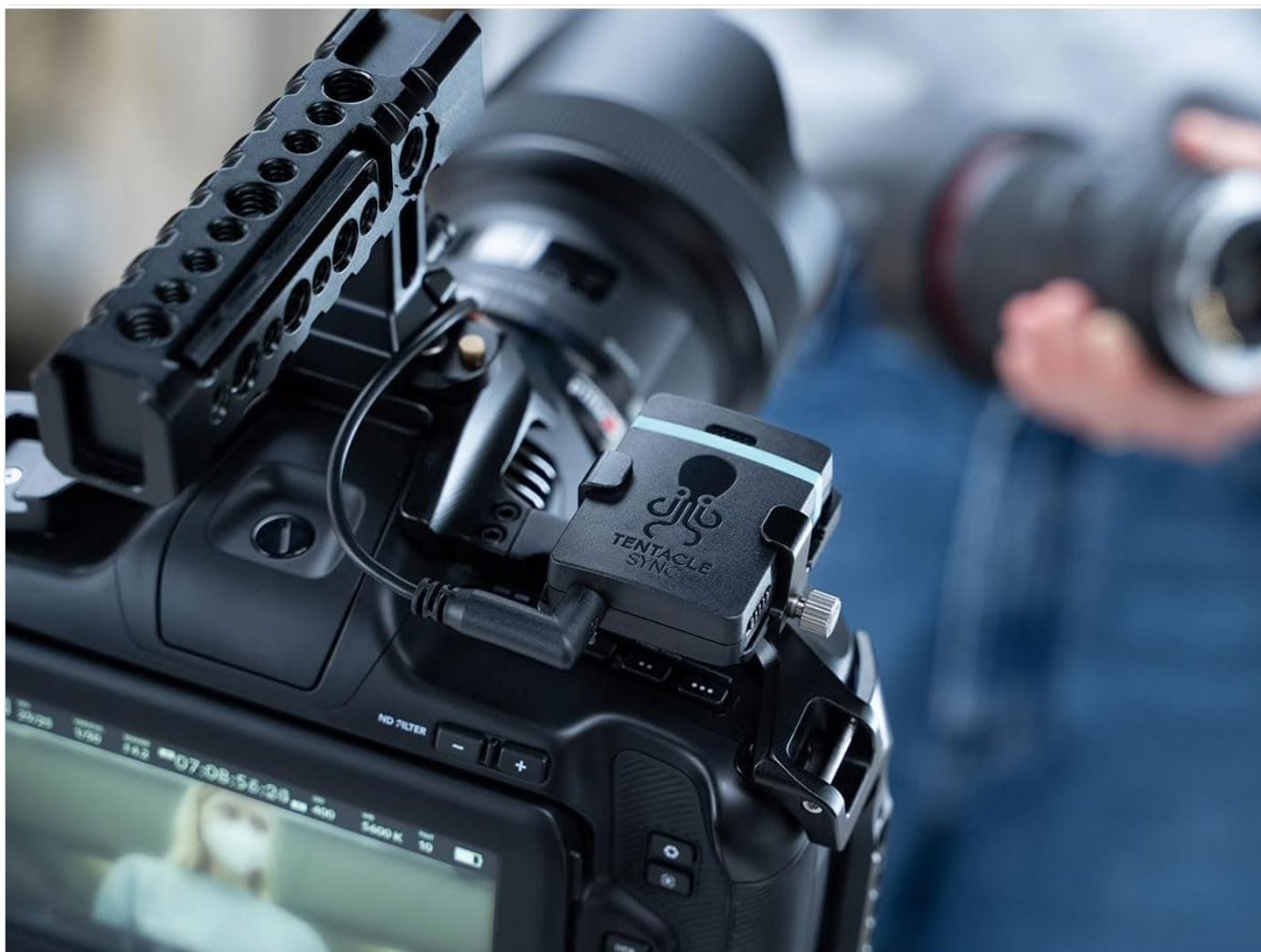
Figure 4.4: The Tentacle Sync E MKII mounted on a professional camera rig, demonstrating its compact size and integration.
