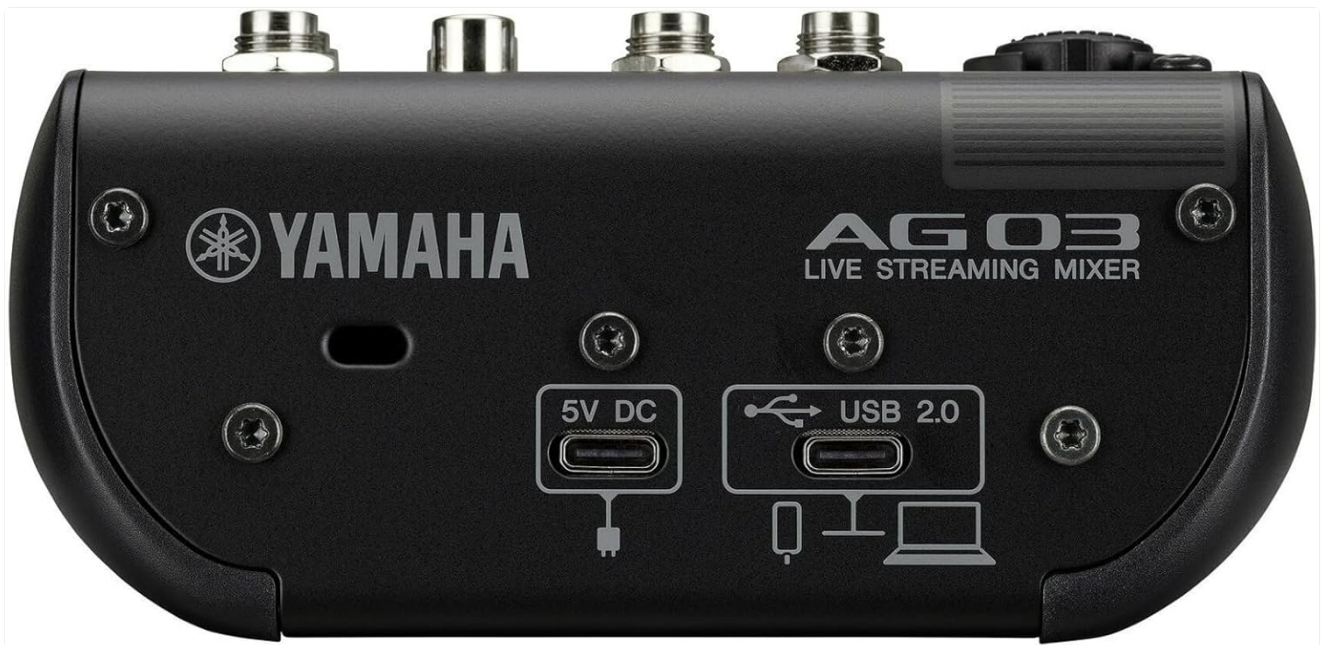
Figure 1: Rear panel of the AG03MK2, highlighting the 5V DC and USB 2.0 connections for power and data transfer.
