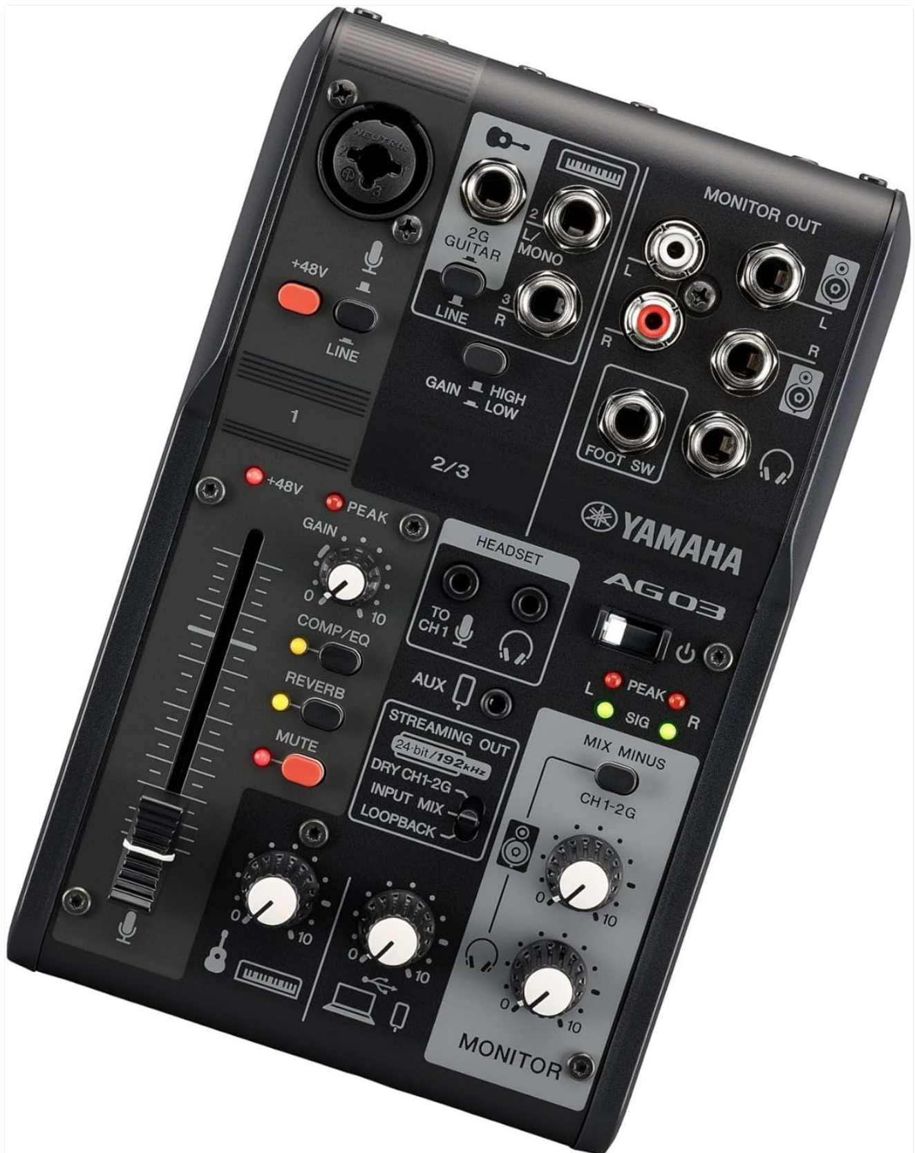
Figure 3: Top panel controls of the AG03MK2, including the main fader, gain knobs, and mute button.
