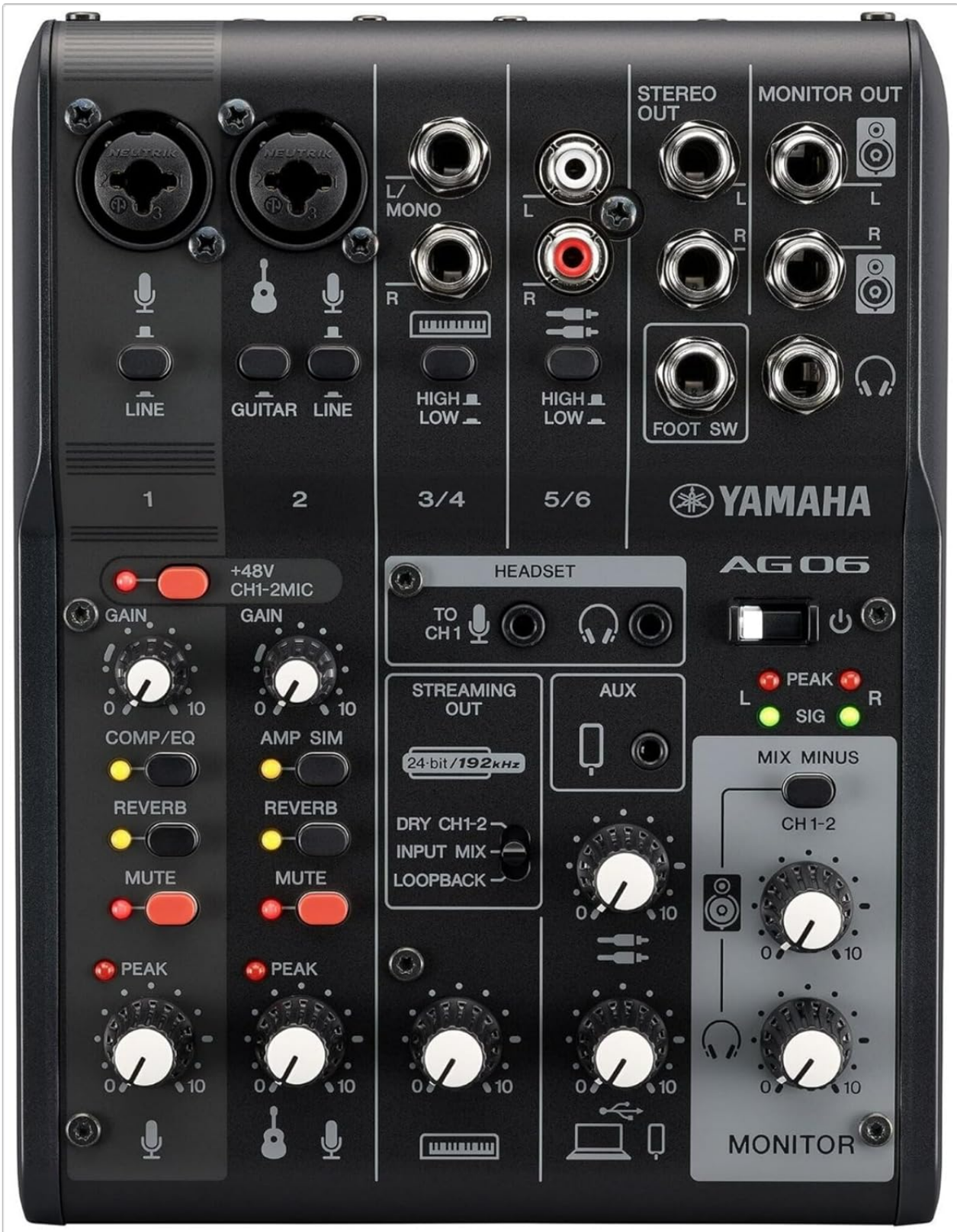
Figure 3.1: Top view of the Yamaha AG06MK2 mixer, showing all controls and inputs/outputs. This image illustrates the compact design and comprehensive control layout.
