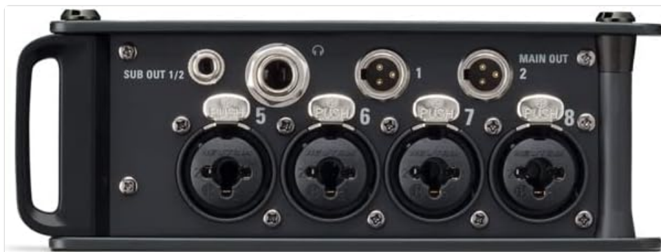
Image: Side view of the Zoom F8n Pro, displaying XLR/TRS inputs 5-8, headphone jack, and main outputs.
