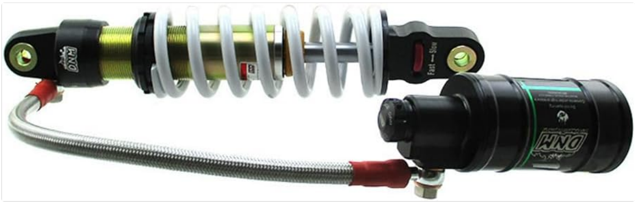
Figure 6.1: View of the rear shock showing the rebound adjustment mechanism (Fast-Slow).
