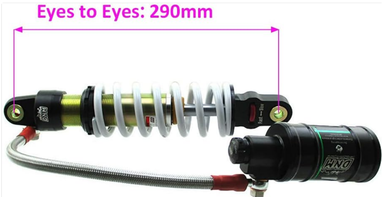
Figure 5.2: Illustration showing the 290mm eye-to-eye measurement of the rear shock.
