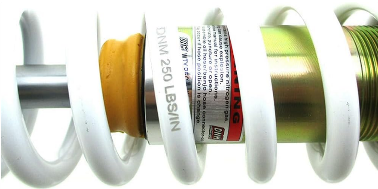
Figure 7.1: Close-up of the shock spring and a warning label indicating high pressure.
