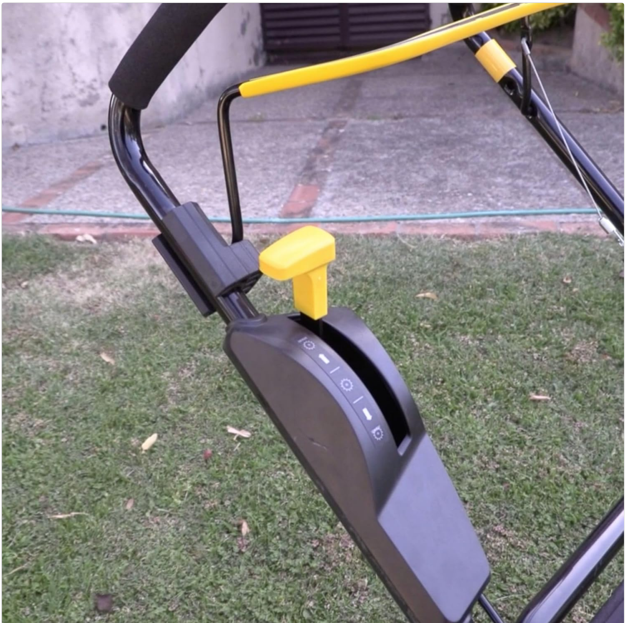
Figure 5: The scarifier in use, demonstrating the position of the depth adjustment lever during operation.
