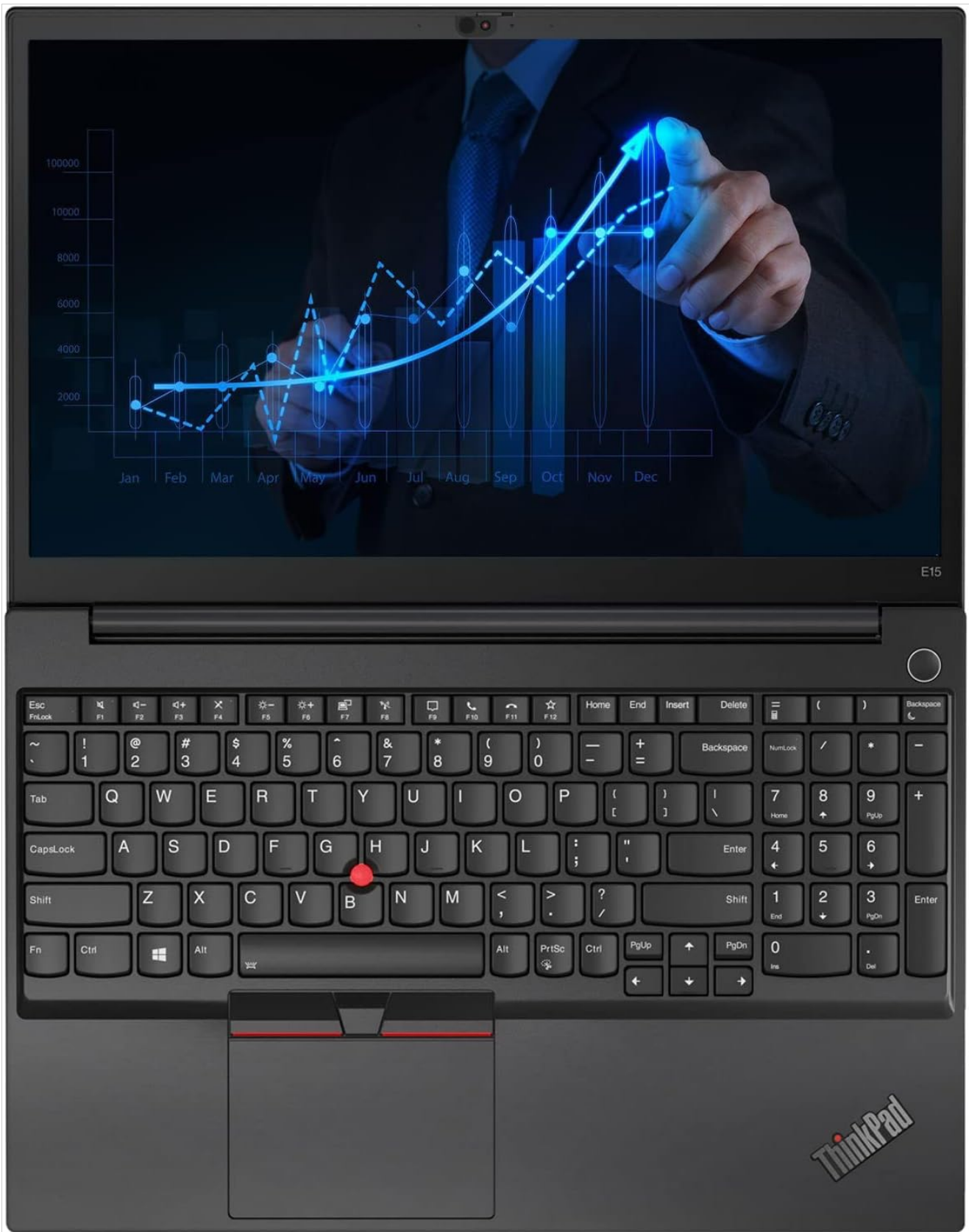
Figure 3.2: Top-down view of the laptop's keyboard, including the numeric keypad, TrackPoint, and trackpad with dedicated buttons.
