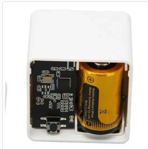
Internal components of the robot switch, including the CR2 lithium battery.
