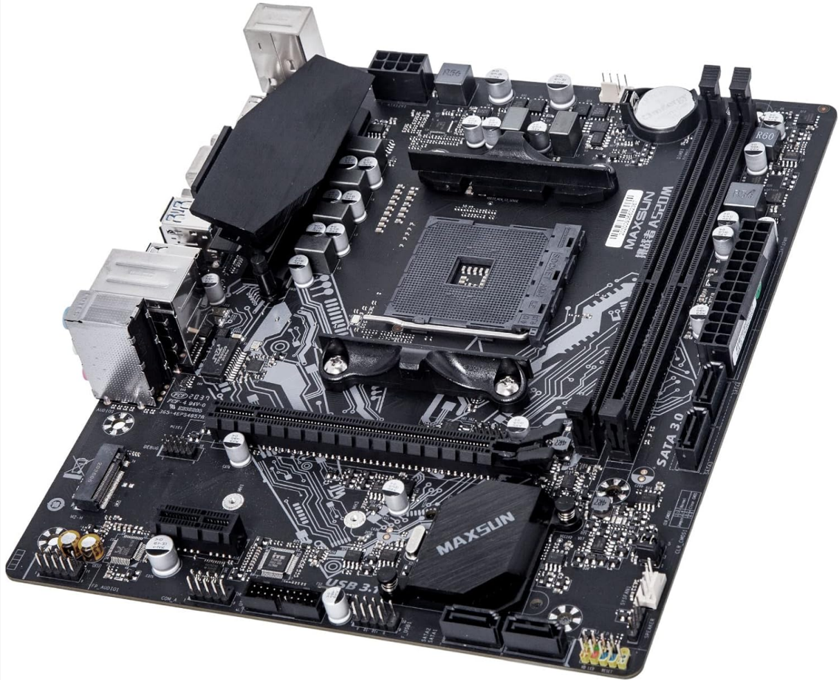
Figure 3.1: Top-down view of the MAXSUN A520M Motherboard, highlighting the CPU socket, RAM slots, and various connectors.
