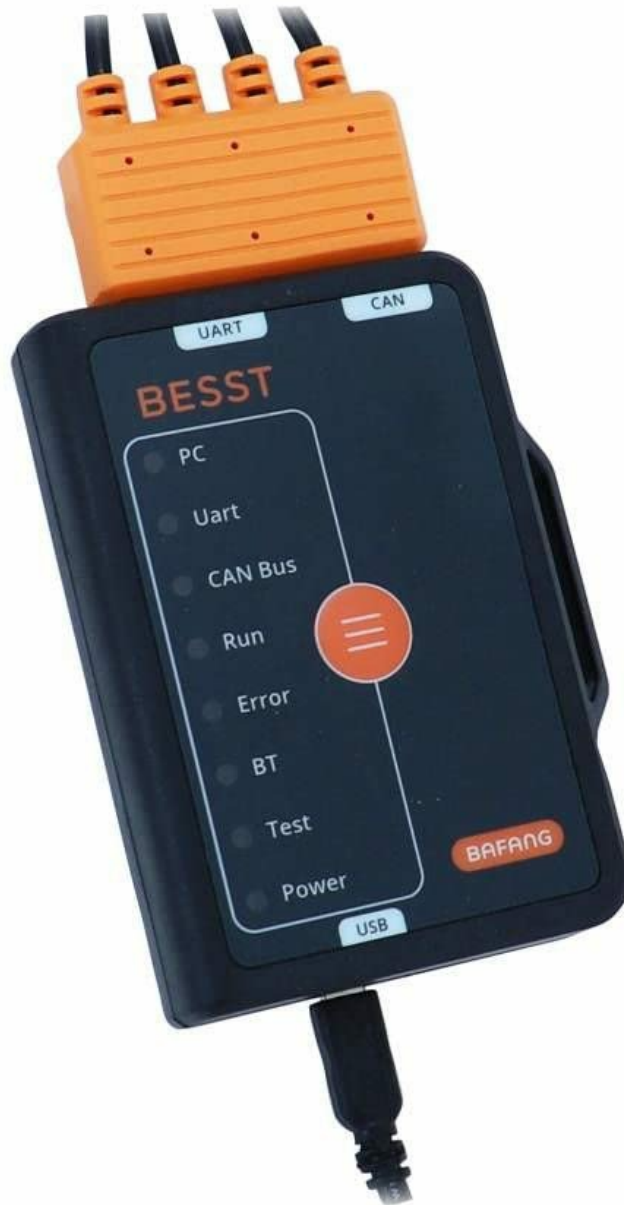
Figure 3: Close-up of the diagnostic tool's indicator lights. These LEDs provide visual feedback on the tool's status: PC (connection to computer), UART/CAN Bus (communication with motor), Run (active operation), Error (fault detected), BT (Bluetooth, if applicable), Test (diagnostic mode), and Power (power supply).
