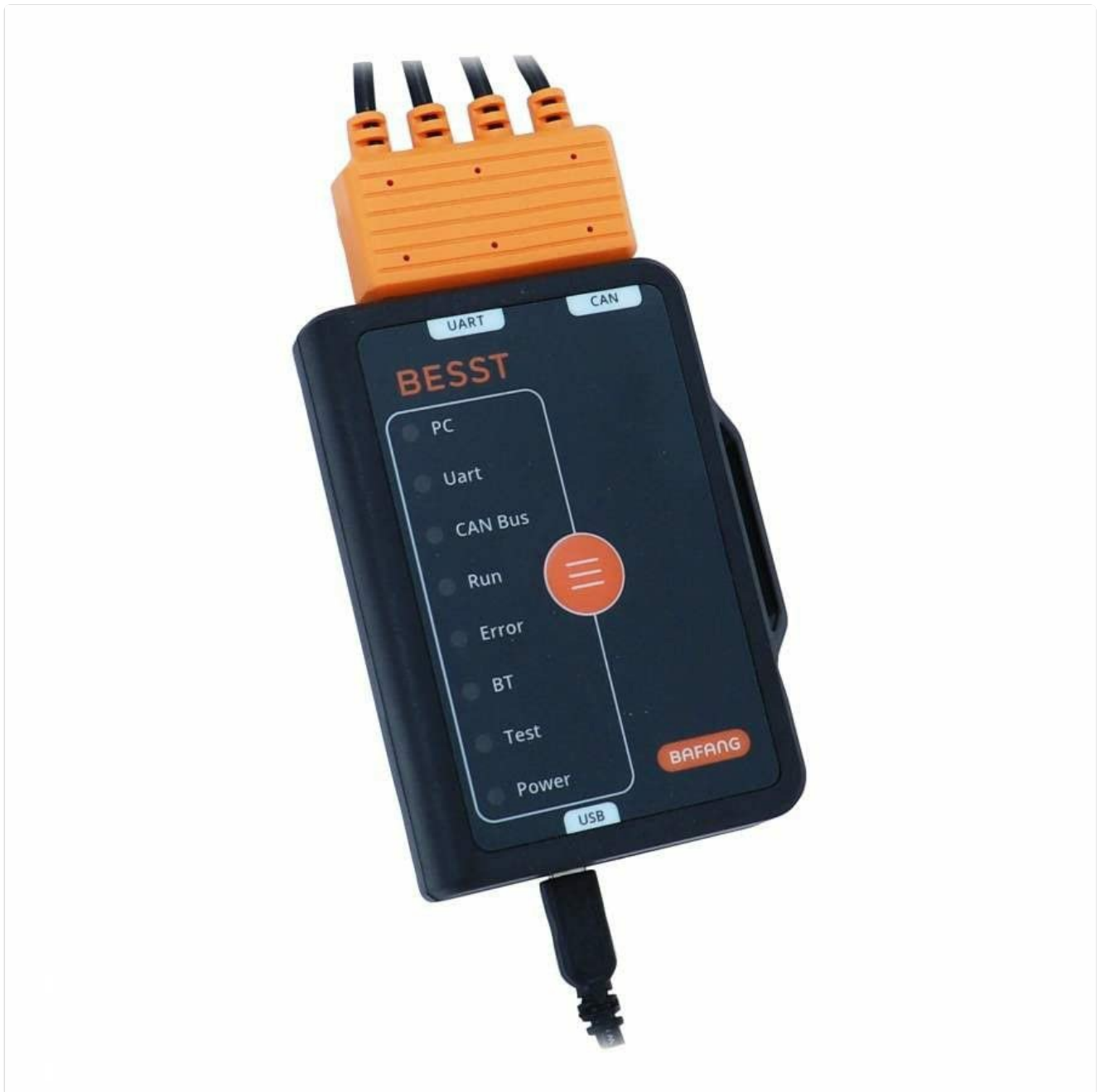
Figure 2: Top view of the diagnostic tool, highlighting the UART and CAN connection ports for different motor types. Proper selection of the port is crucial for establishing communication.
