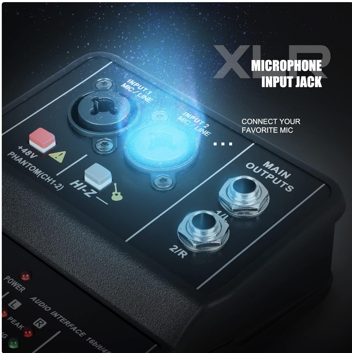
Figure 3: Close-up of the XLR/TRS combo input jacks.
