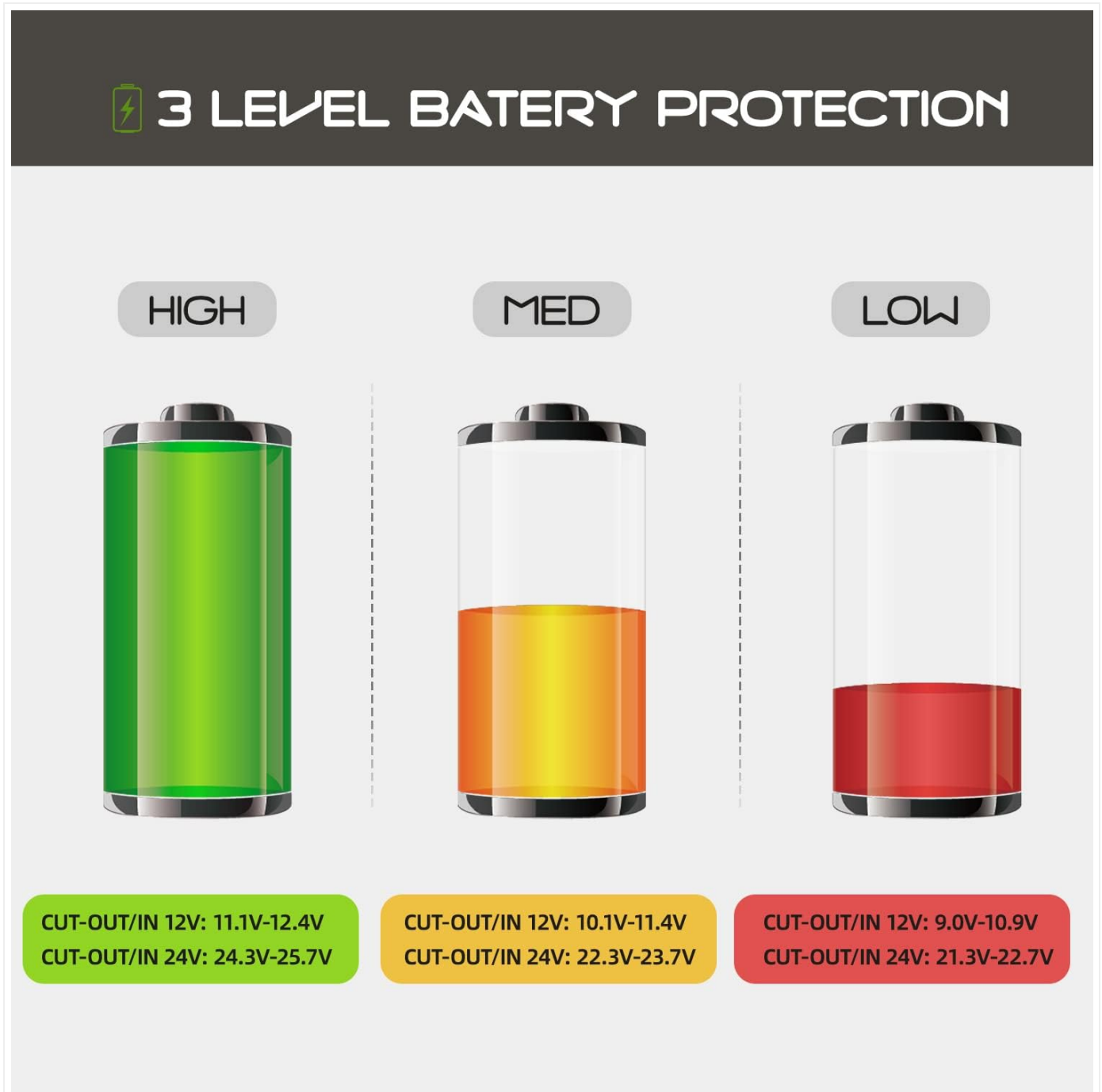
Image: A visual guide to the three battery protection levels (High, Med, Low) and their corresponding cut-off voltages for 12V and 24V systems.
