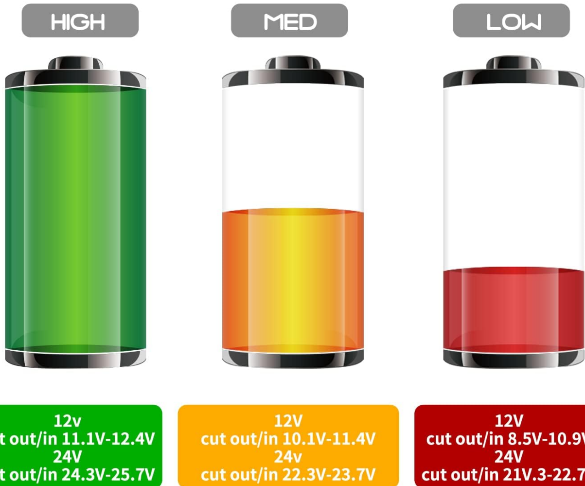
Image: Diagram illustrating the three battery protection levels (High, Med, Low) and their corresponding cut-off voltages for 12V and 24V systems.
