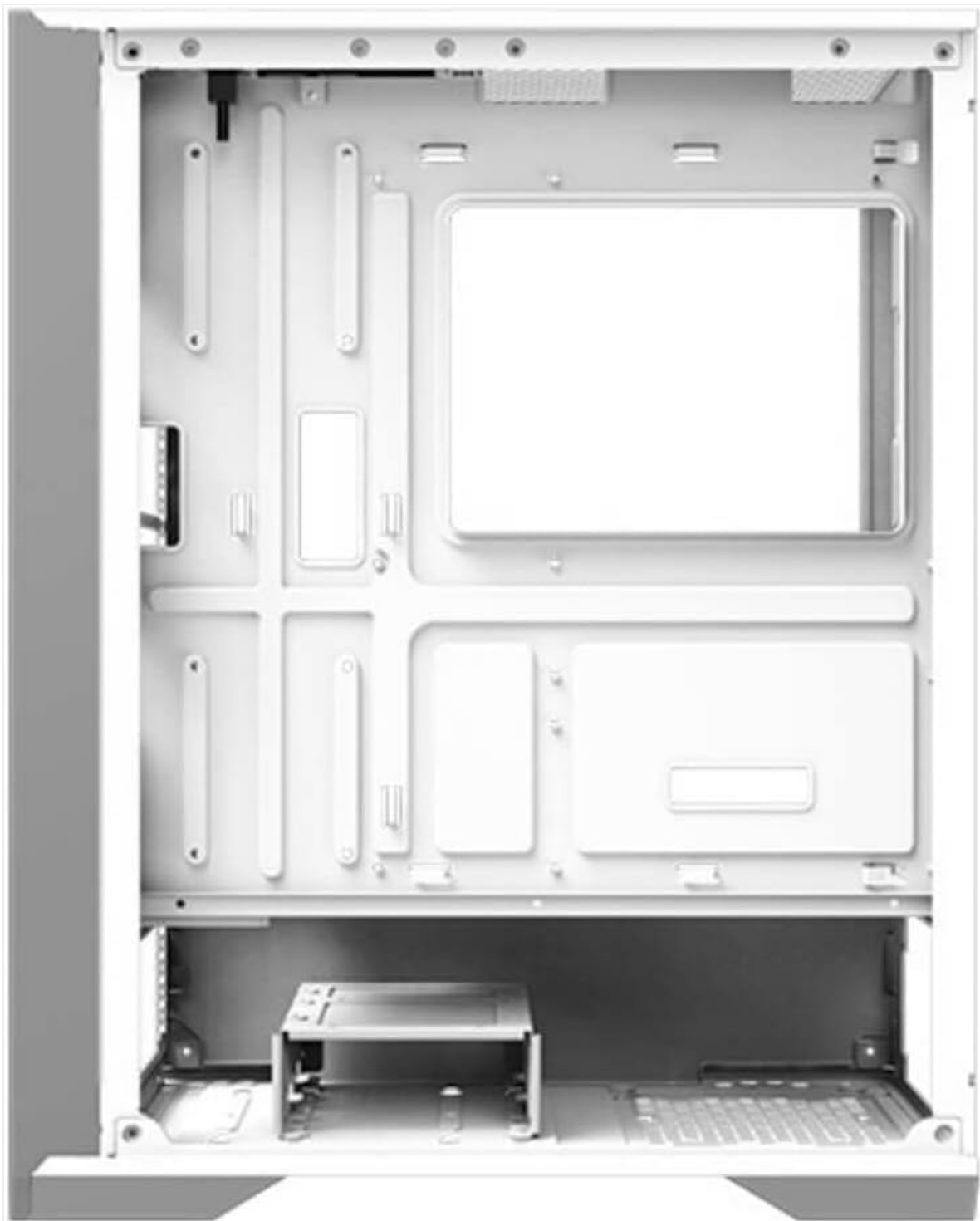
Figure 3.2: Rear interior view, highlighting cable management cutouts and storage drive mounting locations.
