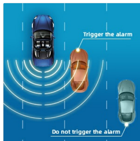
Figure 5.2: Early Warning and Blind Zone Detection Range.
