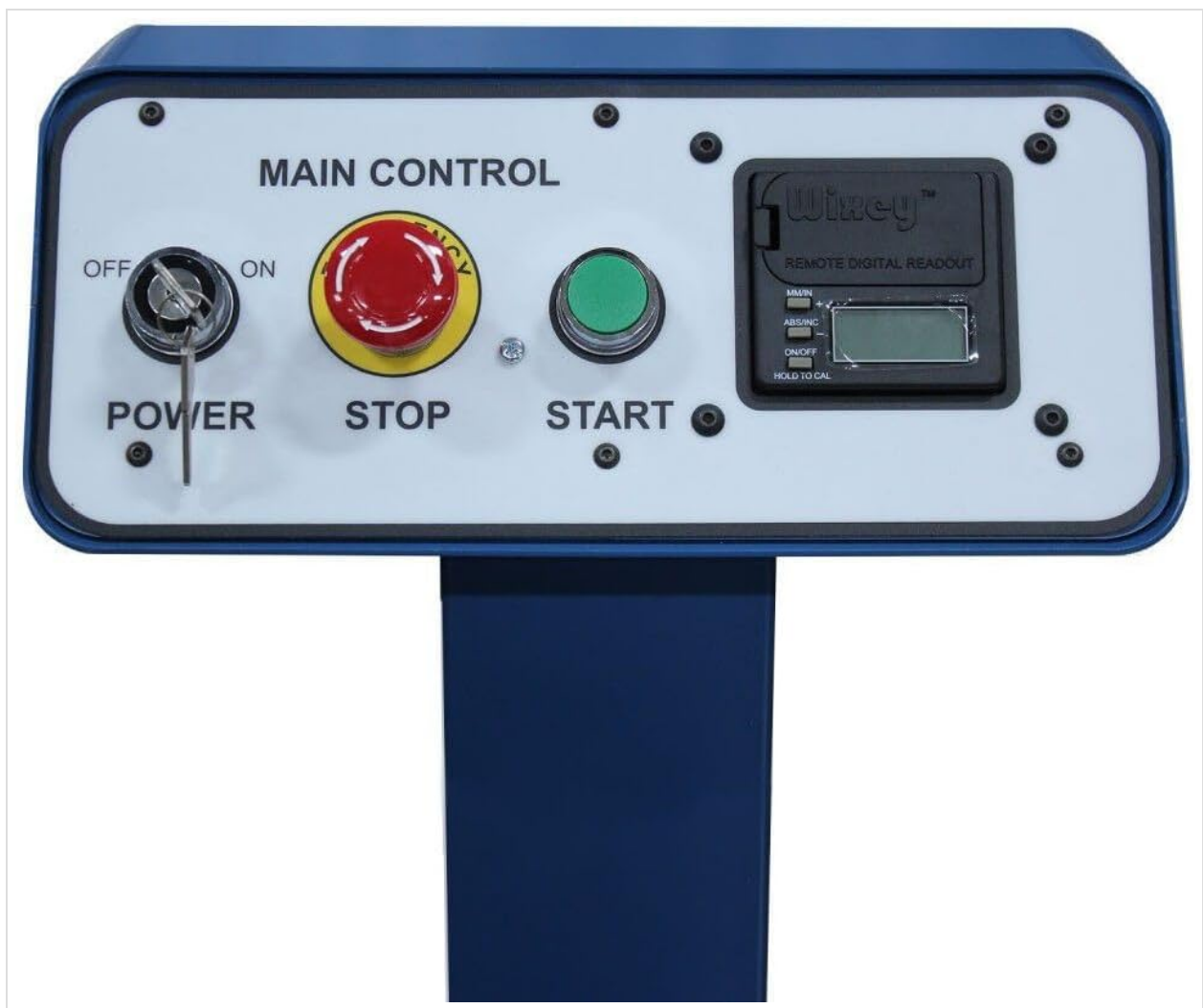
Figure 2: Close-up of the main control panel, featuring power key switch, emergency stop button, start button, and a remote digital readout for precise adjustments.
