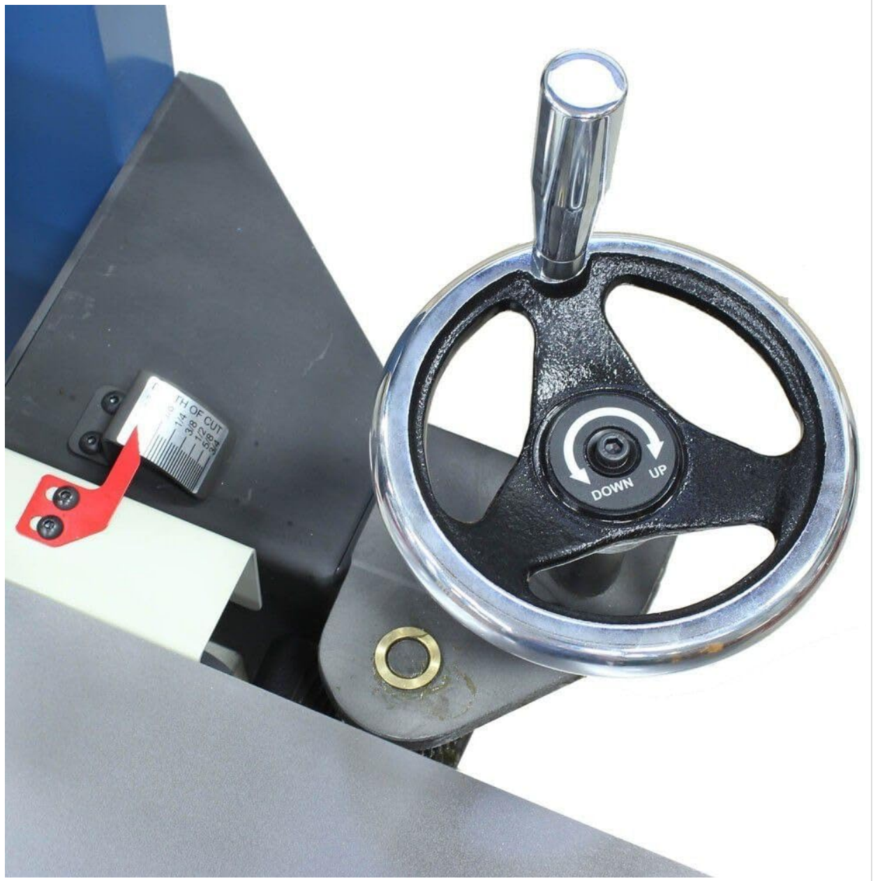
Figure 3: Handwheel mechanism for adjusting the jointer table height, allowing for precise depth of cut settings.
