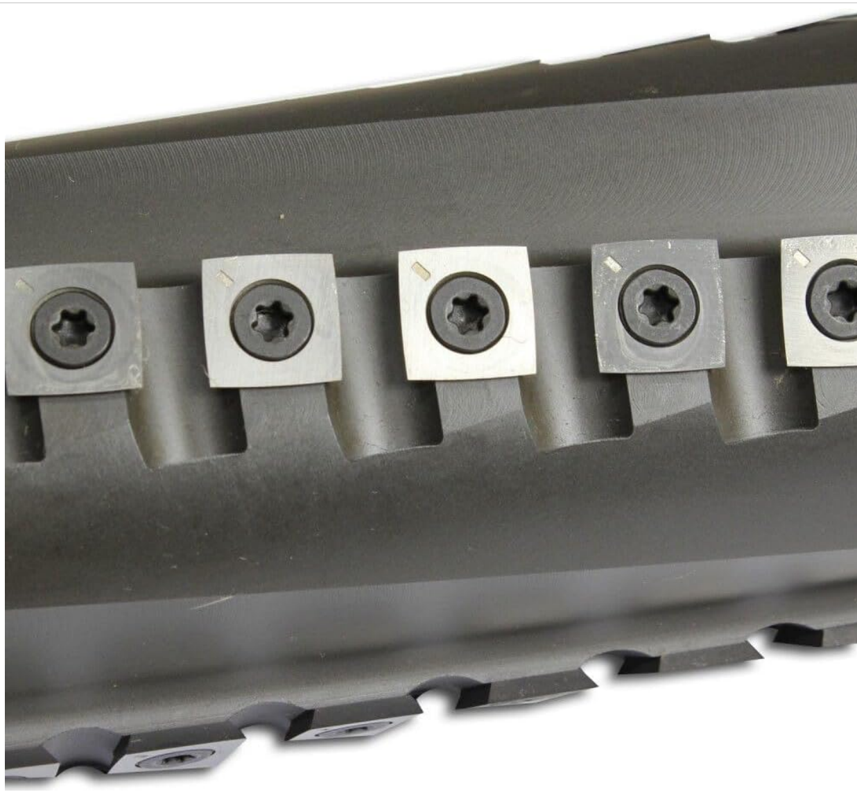
Figure 7: A detailed view of the individual carbide inserts on the helical cutter head, which can be rotated or replaced when dull.
