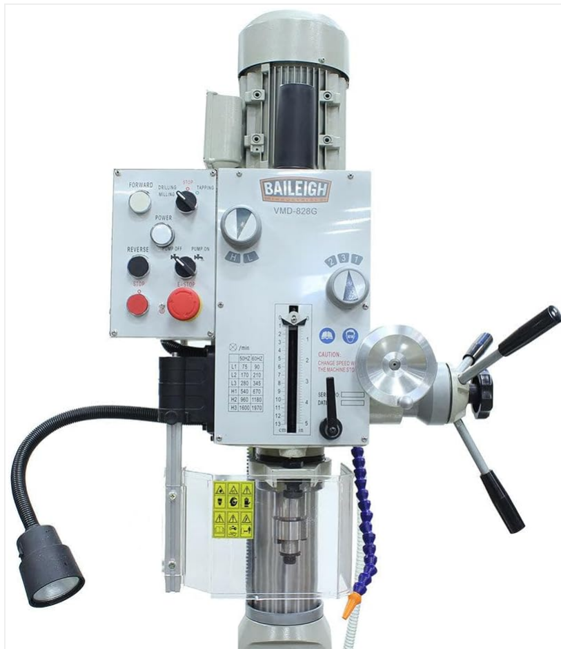
Figure 2: Main control panel with power, direction, and emergency stop buttons.
