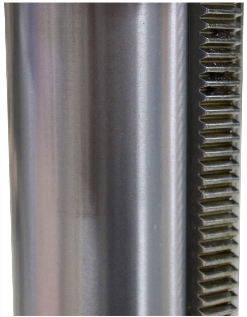
Figure 7: The machine column and rack require regular lubrication to ensure smooth vertical movement.
