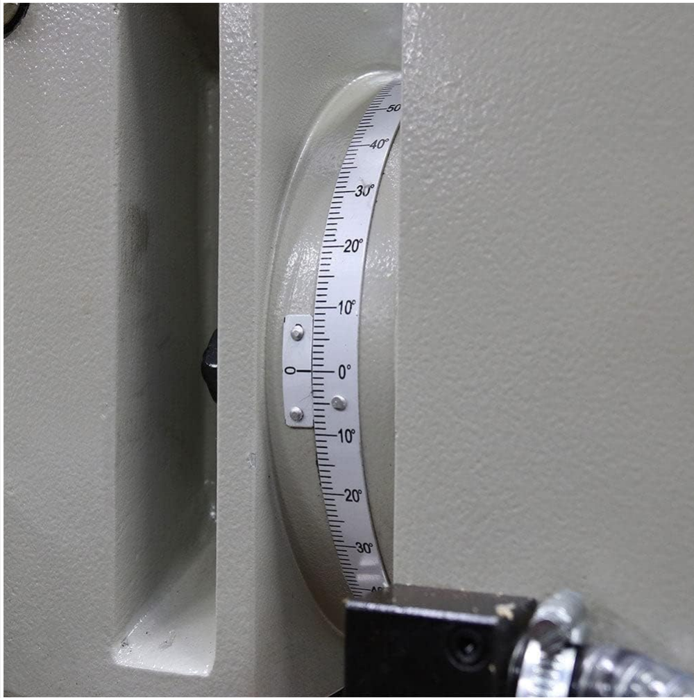
Figure 6: Angle scale for tilting the machine head.
