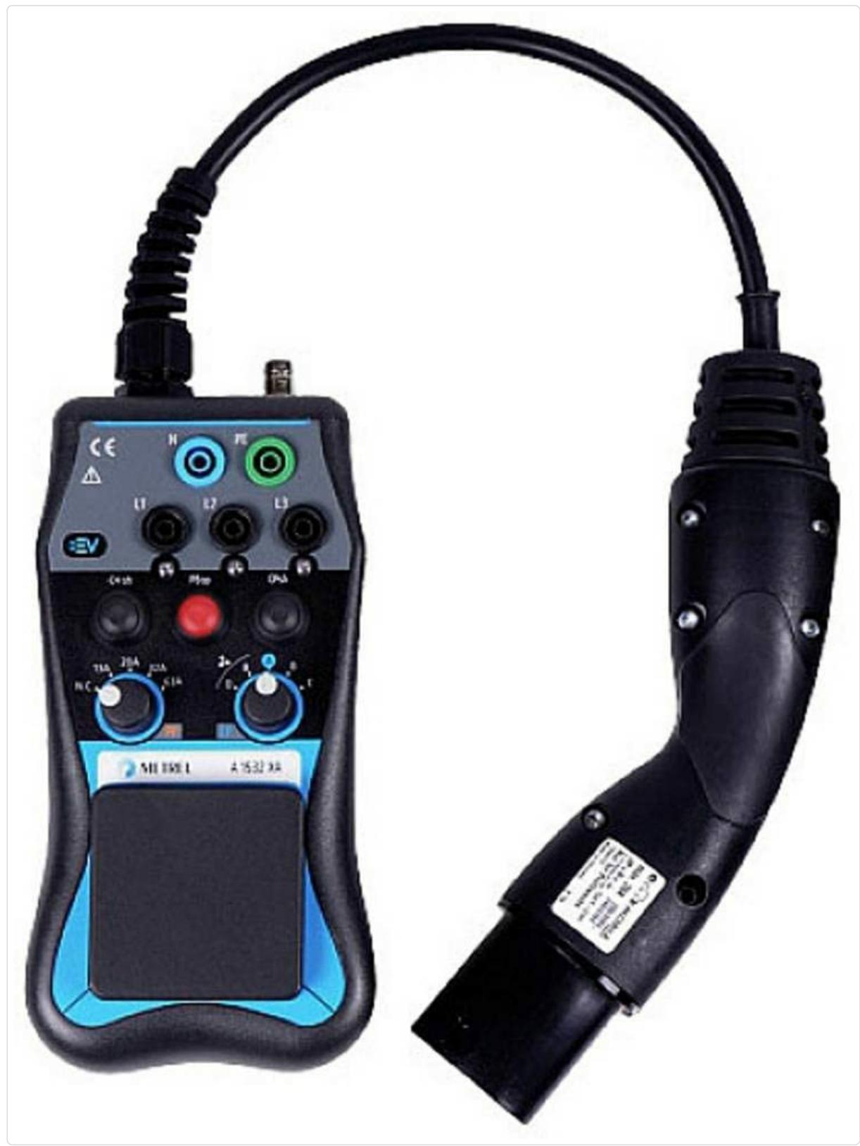
An image showing the Metrel 1532 XA EVSE Charging Station Adapter. The device consists of a main testing unit with various input ports (H, N, PE, L1, L2, L3), control dials, and buttons, connected by a cable to an EV charging plug. The main unit is black and blue with clear markings for connections and controls.
