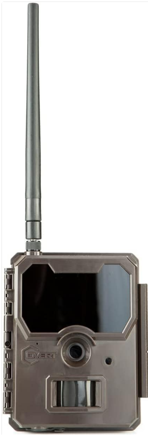
Front view of the Covert WC20-V cellular game camera, showing the lens, sensors, and attached antenna.
