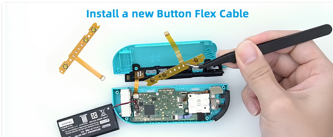
Image: A hand using precision tweezers to carefully place the new button flex cable onto the circuit board inside the opened Joy-Con controller.
