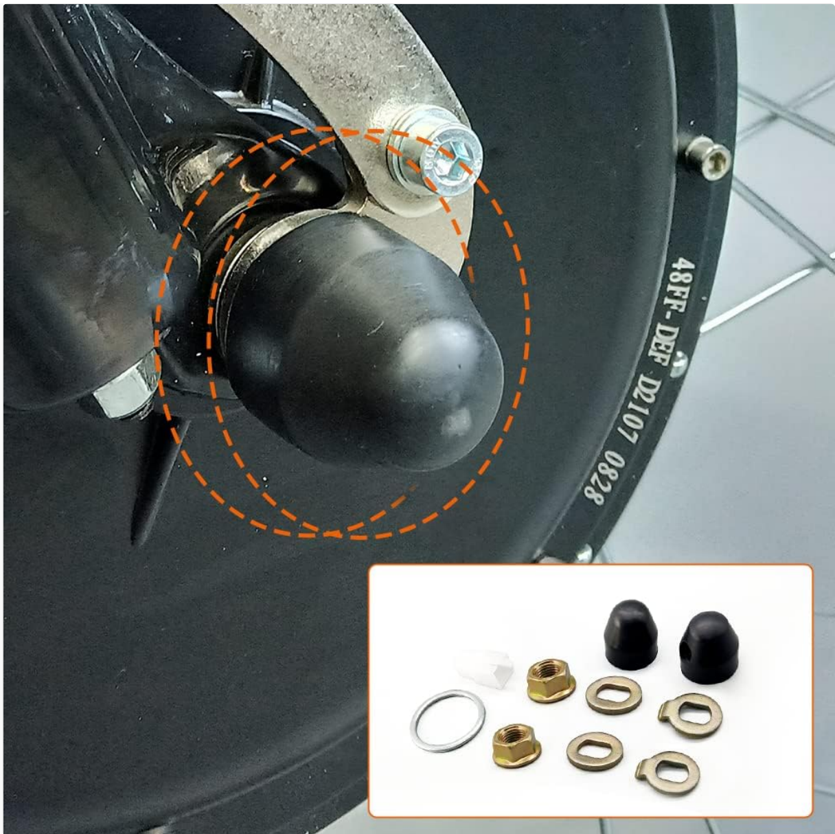
Image 4.2: The complete set of components and a detailed view of a protective cap properly installed on an e-bike hub motor axle.
