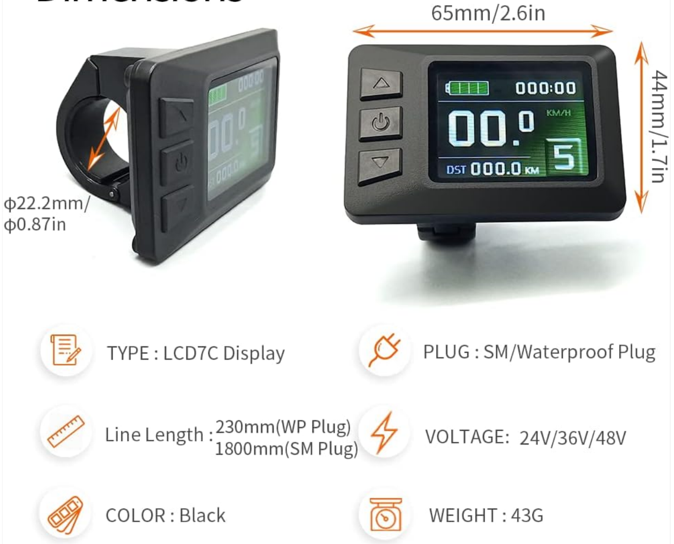
Figure 3: KT-LCD7C display dimensions and key specifications.
