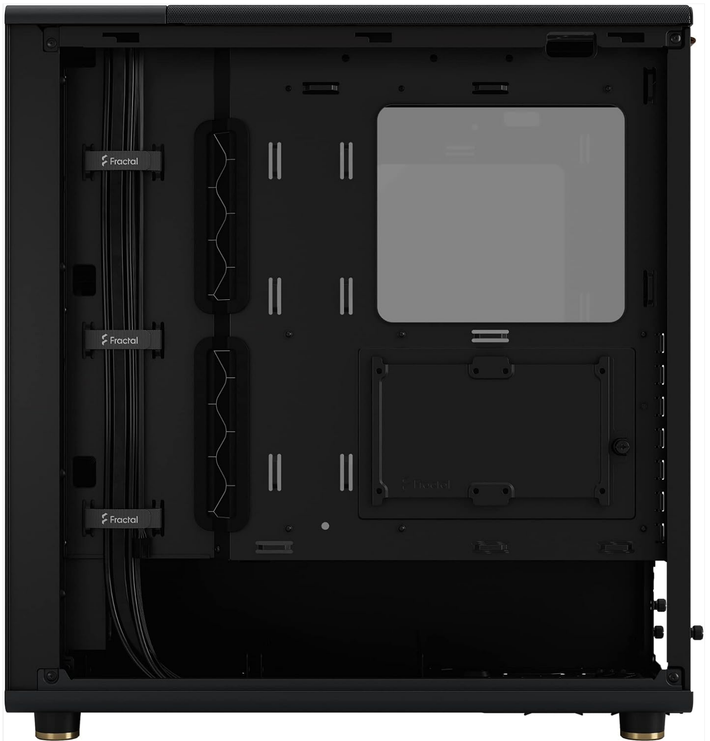
Figure 6: Rear view of the case interior, illustrating the cable routing channels and Velcro straps for efficient cable management.
