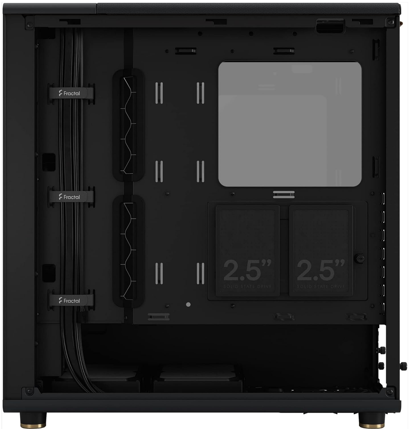
Figure 5: View of the rear side of the motherboard tray, showing the dedicated 2.5-inch drive mounts for SSDs.
