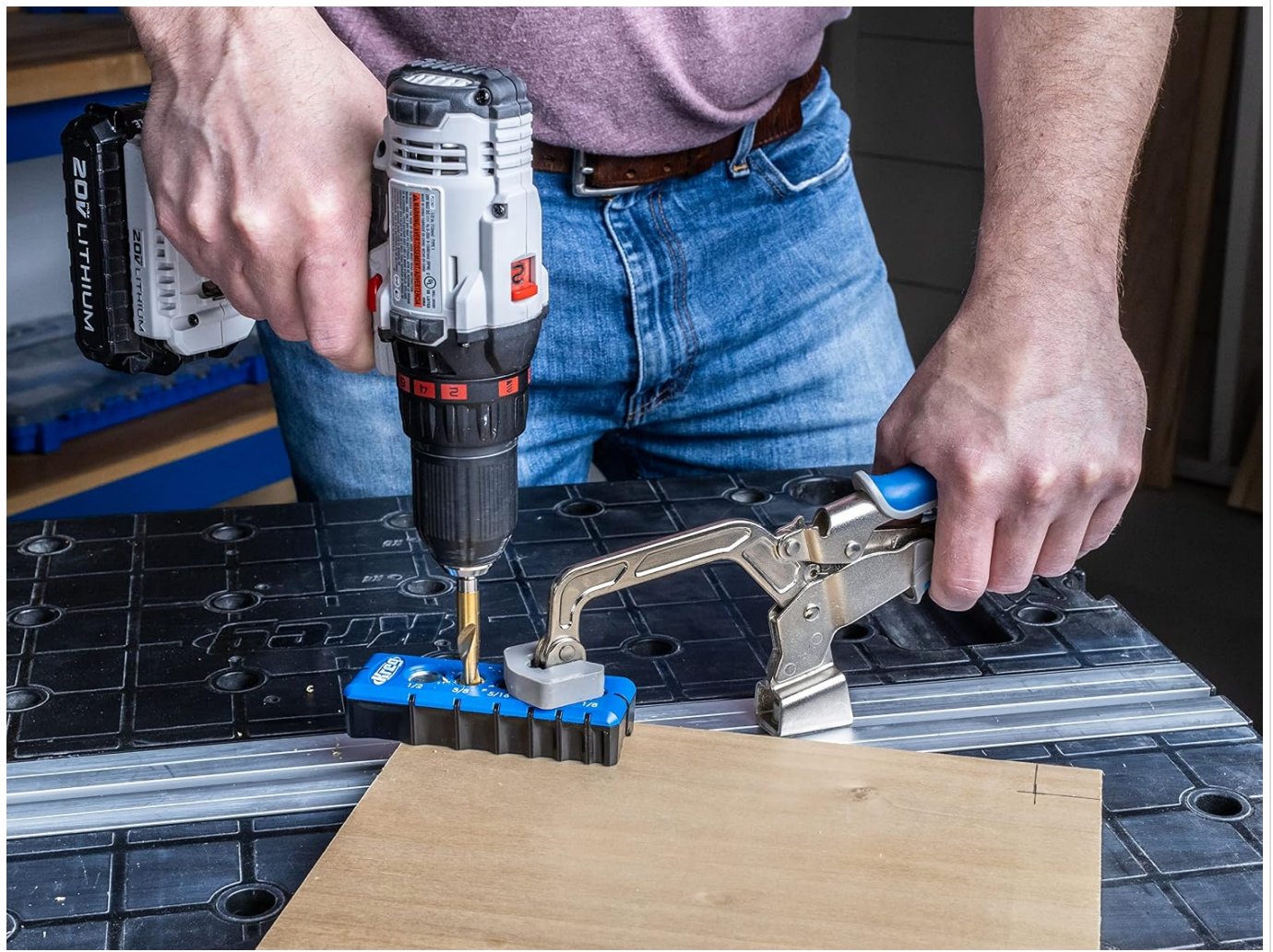
A user utilizing the Kreg Portable Drilling Guide with an additional clamp for enhanced stability while drilling.
