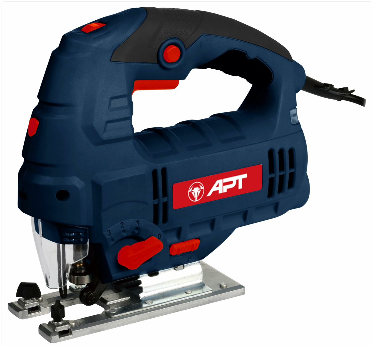
Figure 1: Total 800W Jigsaw Model DW07455. This image displays the main unit, highlighting its 800W power, adjustable base plate for up to 45-degree bevel cuts, and cutting capacities of up to 110mm for wood and 10mm for metal. It also indicates 6 variable speed settings and a B-type blade compatibility.
