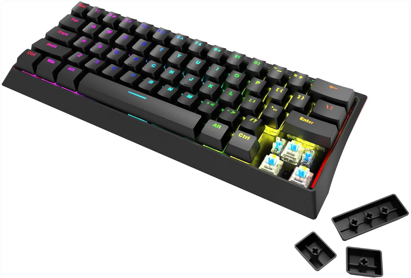
Figure 4: Detail of the Marvo KG962 keyboard, highlighting the blue mechanical switches and removable keycaps.
